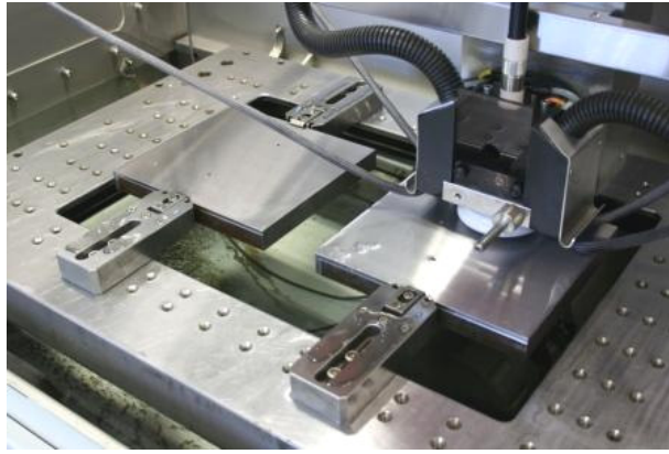
Workpieces fixation by means of 4 rulers WZ150L
